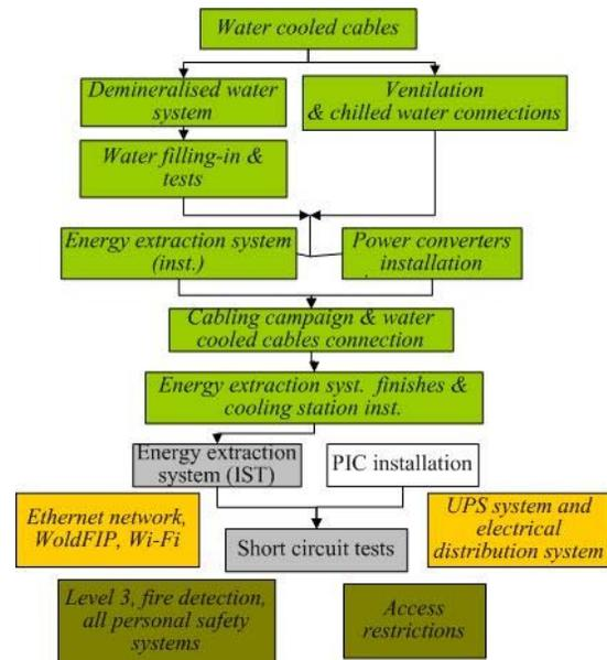
Figure 1: Requirements of the short circuit test: Green = installation activities, Grey = individual system tests, White = interference with other systems, Yellow = general services, Khaki = access and safety
