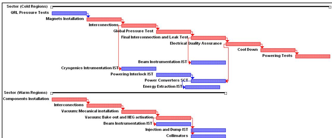
Figure 2: IST dependencies with the activities on the critical path and in between ISTs. Red bars correspond to installation activities and blue bars to IST (bar lengths do not represent the precise duration of the activities)
