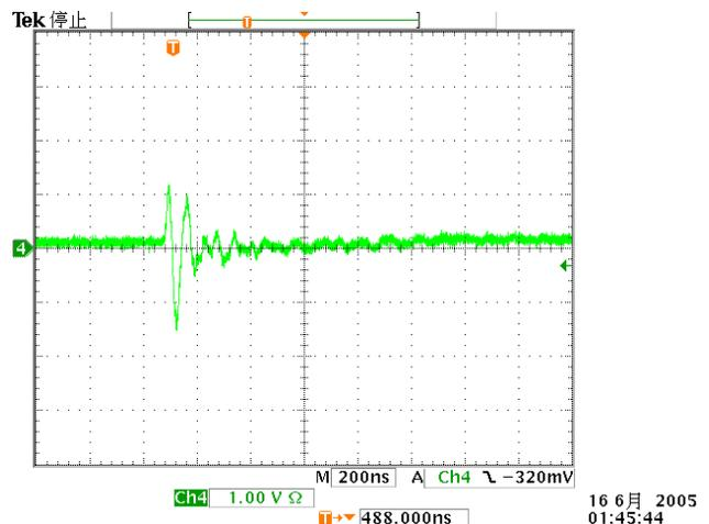
Figure 5: Noise picked up after EMI wrapper enclosed.
