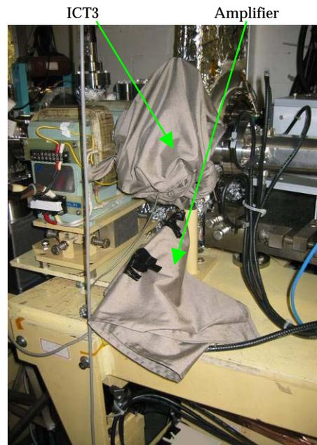
Figure 5: EMI wrapper enclosed the ICT3 & amplifier.
