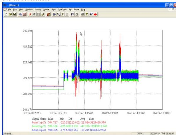
Figure 8: Signal after EMI reduction.
