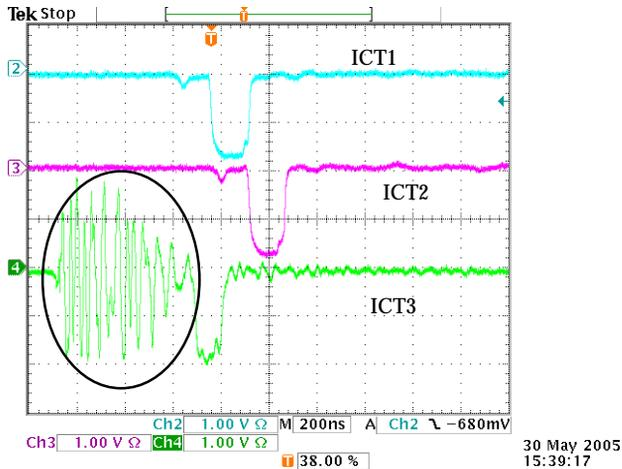
Figure 3: The signals measured by ICTs.
