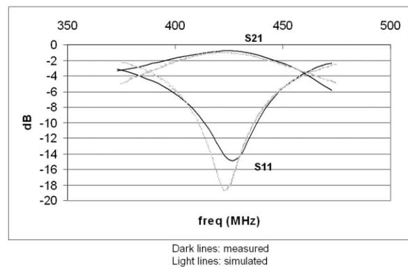
Figure 3: Alumina match measurement.
