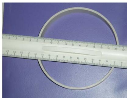
Figure 1: Large-diameter ceramic ring sample made of BST-MgO (BSM) ferroelectric. The ring diameter is of 110 mm and the ring thickness is of 2.8 mm.
