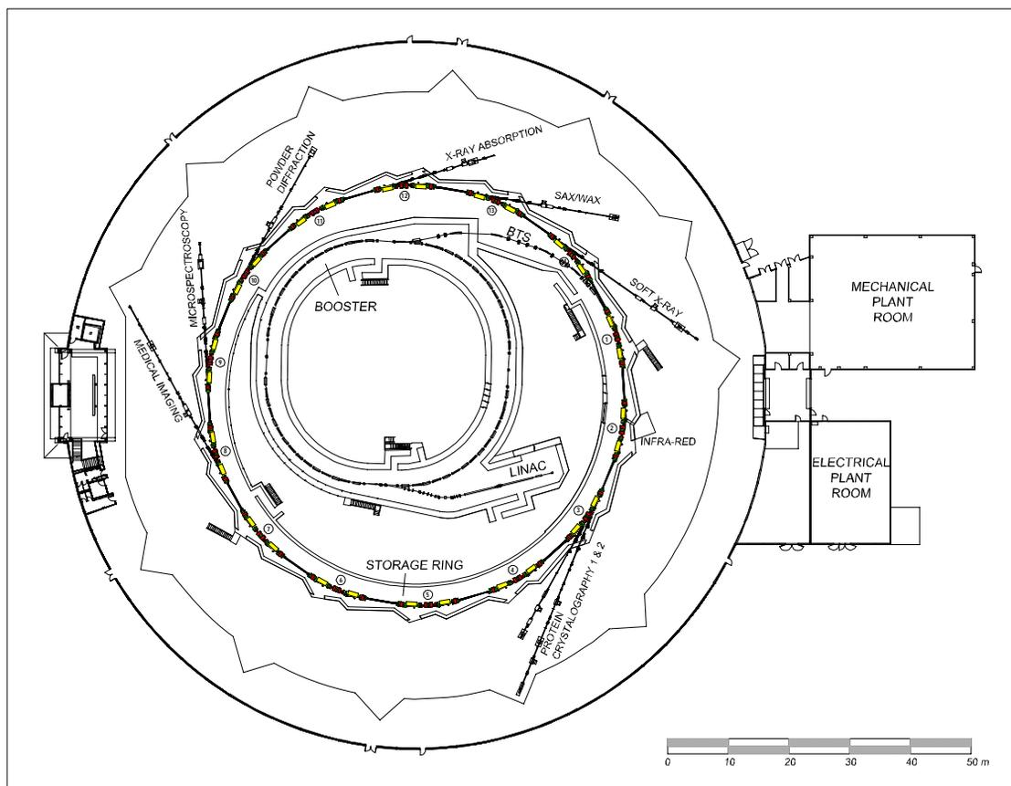
Figure 6: Layout of the Australian Synchrotron
