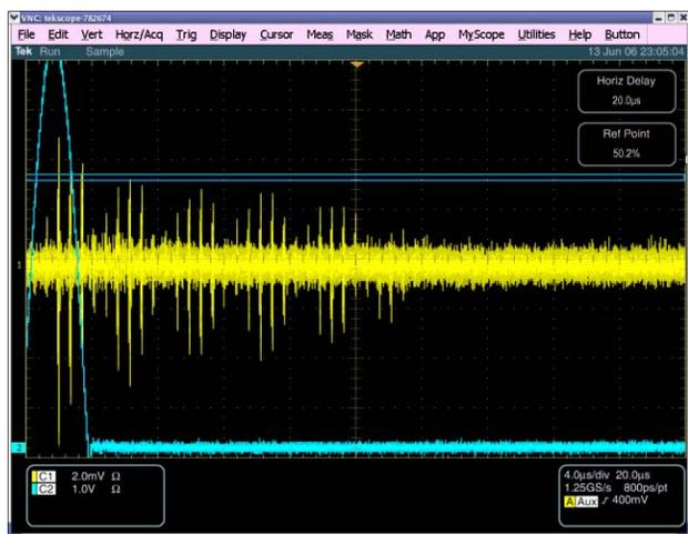
Figure 5: A trace showing the first ~30 turns in the storage ring.
