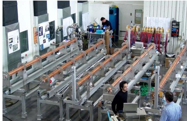
Figure 1: Linac functional units. In the front: accelerating structures during tuning, in the back left: MEBT; in the back right : bunching section during assembly.
