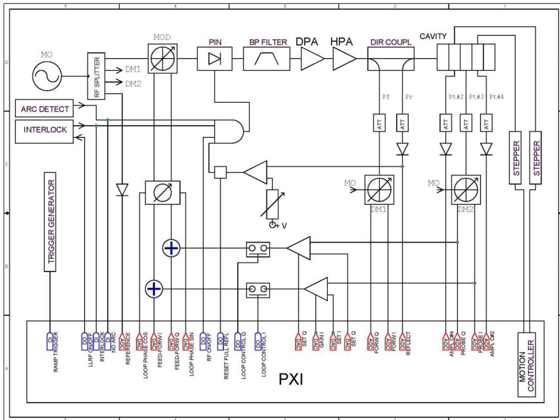
Figure 4: ASP booster LLRF diagram.
