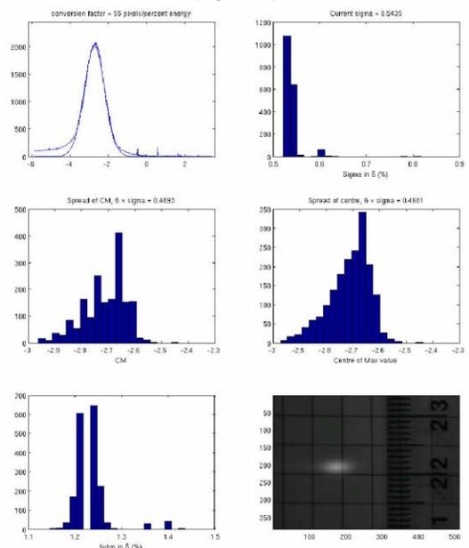
Figure 2: Energy, energy spread and energy stability measurement as performed by ASP for single bunch mode.
