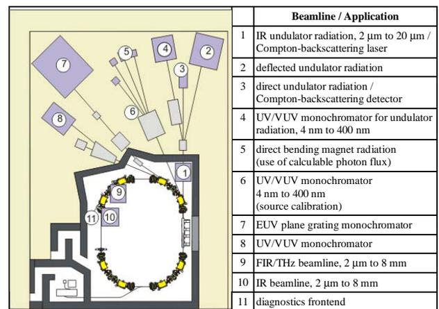
Figure 2: Planned beamlines and experimental stations at the MLS.
