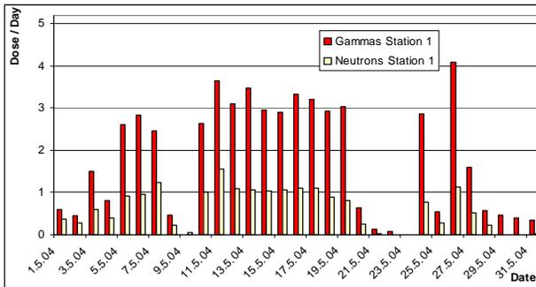
Figure 6: Gamma and neutron dose per day in  $[\mu\text{Sv}]$  at station 1 in May 2004
