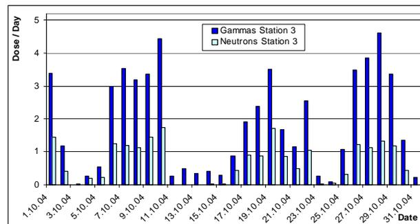
Figure 9: Gamma and neutron dose per day in  $[\mu\text{Sv}]$  at station 3 in October 2004
