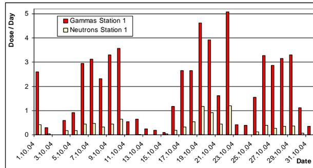
Figure 8: Gamma and neutron dose per day in  $[\mu\text{Sv}]$  at station 1 in October 2004
