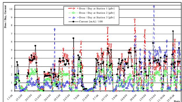
Figure 5: Current and total dose per day measured at three stations
