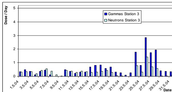
Figure 7: Gamma and neutron dose per day in  $[\mu\text{Sv}]$  at station 3 in May 2004
