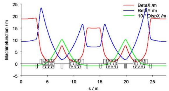
Figure 3: Machine functions for 100 nmrad emittance
