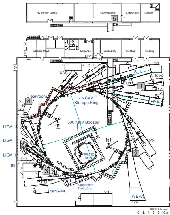
Figure 1: ANKA Facility with Radiation Detector Stations 1-5
