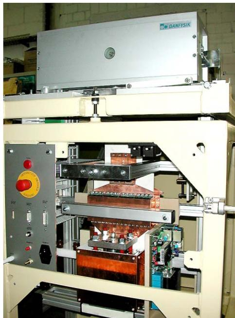
Figure 1: Storage ring injection kicker, magnet upper, pulser below, variable tuning inductance centre.
