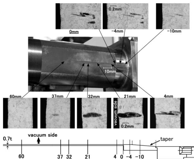
Figure 2: Injection chamber damaged by electron beam.
