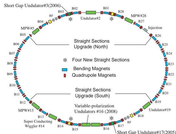
Figure 1: Reconstructed area for the straight sections upgrade of the PF ring.
