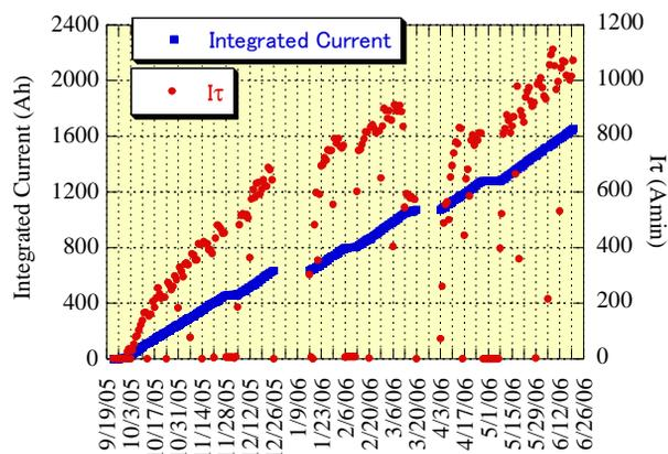
Figure 3: Integrated current and the recovery of the beam lifetime during 9-month operation after the recommissioning. or about 8 hours at 450 mA.
