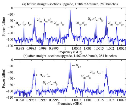
Figure 4: Betatron sidebands observed in the usual partial filling changed from the vertical (a) to the horizontal (b) after the upgrade.
