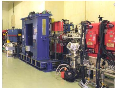
Figure 2: Example of extension of a straight section. A free space of about 1.5 m has been created between the MPW#5 and the quadrupole doublet on this side.
