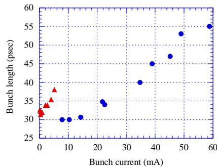
Figure 5: Comparison of the bunch lengthening before (triangle) and after (circle) the reconstruction.
