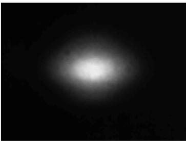
Figure 4: Intensity distribution of the light beam at the afocal system.
