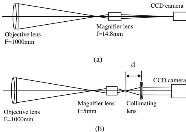
Figure 1: Focusing system (a) for the observation of the beam position and afocal system (b) for the observation of beam angle.
