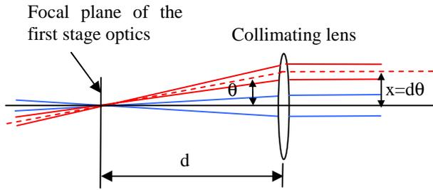
Figure 2: Collimating section in the afocal system.
