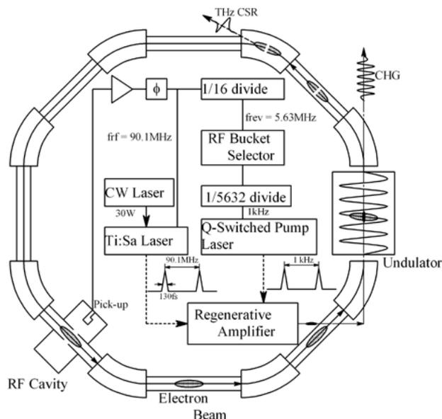
Figure 1: Schematic drawing of the laser bunch slicing system.
