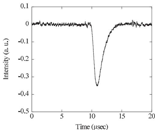
Figure 4: Detector output signal (negative) for individual terahertz pulse.
