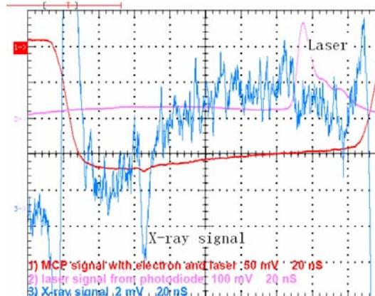
Fig. 2: Oscilloscope trace showing the laser pulse, the signal obtained from MCP, and the detected X-ray signal.
