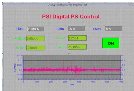
Figure 5: Digital Controller tested on EPICS.
