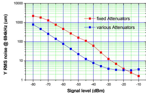
Figure 3: Libera resolution test @ CW mode
