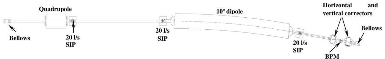
Figure 5: the vacuum layout of the unit cell of the booster synchrotron
