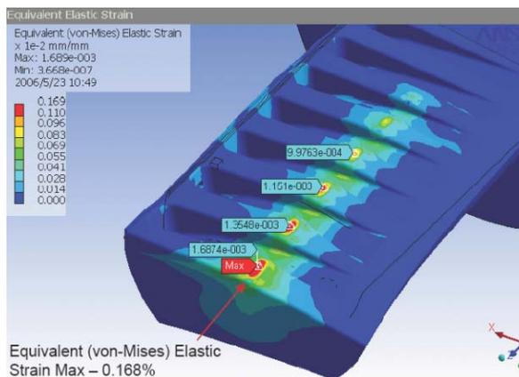
Figure 3: the equivalent von-Mises strain for the critical absorber (Glidcop®).
