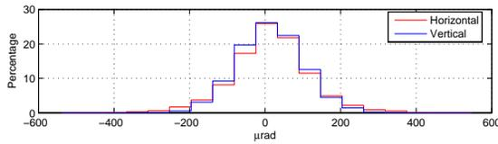
Figure 6: Histogram of the distribution of the strength of the correctors for 200 sample cases, for correcting a realistic distribution of errors.
