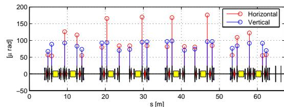
Figure 5: Distribution of the RMS values of the correctors, for 200 sample cases, for correcting a realistic distribution of errors.
