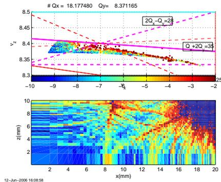
Figure 4: Dynamic aperture and frequency map including the effect of the multipoles.
