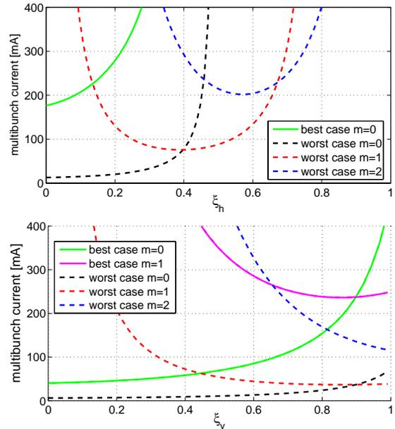
Figure 7: multibunch threshold current of different modes vs. normalized chromaticity for both cases and both planes
