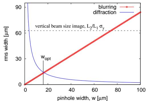
Figure 3: Blurring and diffraction effects as a function of the pinhole width,  $w$ . The dotted line shows the rms vertical beam size considering  $L_2/L_1 = 2$ .
