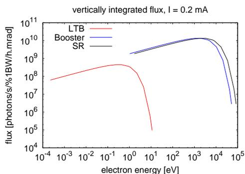
Figure 1: Fluxes along in the injector and SR for a beam current of 2mA.
