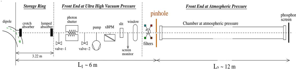
Figure 4: Sketch with the required components to be installed in the XSR [3]. Distances are not to scale.
