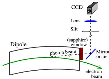
Figure 2: VSR schematic layout in an injector dipole. The mirror reflects the light 90° down or up.
