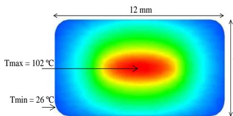
Figure 5: Temperature distribution in the XSR vacuum window. Courtesy of B. Calcagno [5].
