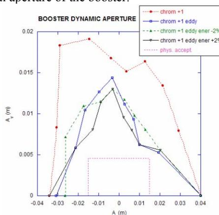
Figure 4: Booster dynamic aperture with  $\zeta_{x,y}=+1$ , with eddy currents at the dipole and off-energy particles
