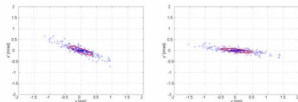
Figure 2: Transverse phase space at linac exit in single bunch mode
