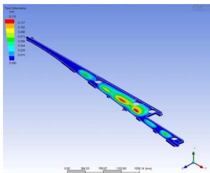
Figure 4: Simulation of the deformation on the lower half of B1 chamber due to the evacuation.
