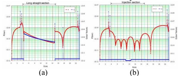
Figure 6: Pressure profiles for the sections of LS-ID (a) and of LS-Inj (b). The outgassing rate and the pressure are illustrated by blue lines and red lines, respectively.
