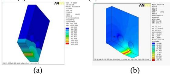
Figure 5: Simulation of the thermal distribution on the downstream Al absorber with interior cooling in cases of irradiation surfaces with (a) saw-tooth structure, and with (b) incline surface.
