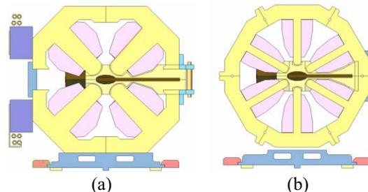
Figure 3: Cross section views of a B-chamber with a Q-magnet (a), and a S-magnet (b).
