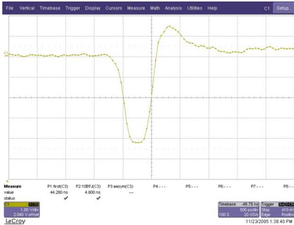
Figure 3: The performance of Kentech - PFN module. The 500ps square pulse (FWHM) signal is displayed by a wideband digital oscilloscope, SDA-6000A.
