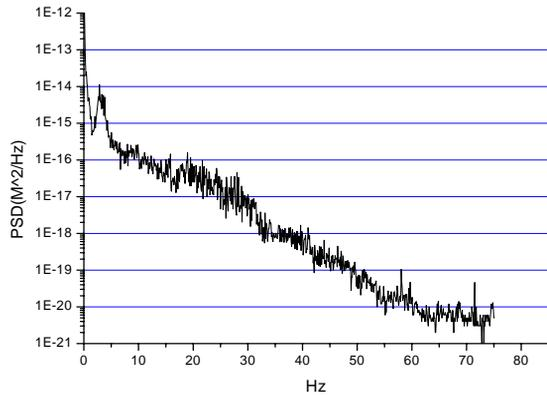
Fig. 2: A typical power spectrum density of ground vibration in vertical direction.
