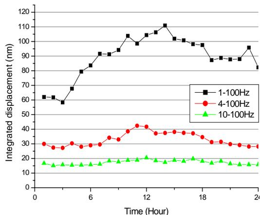
Fig. 6: Vertical vibrations near the TLS tunnel.
