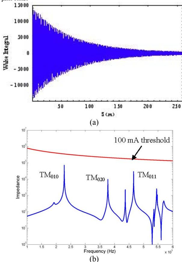
Figure 3: (a) Longitudinal wake integral and (b) longitudinal impedance of a single-cell cavity with a thin waveguide damper.
