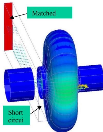
Figure 2: Power density and vector electric field plot of the TM<sub>010</sub> mode in the cavity and in the waveguide damper. The red color represents maximum power loss, while blue is little or no loss.
