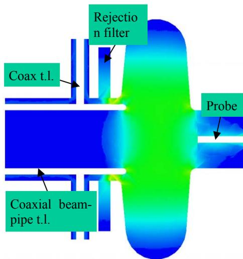
Figure 1: Magnitude of electric field of the TM<sub>010</sub> mode in a KEK-type deflecting cavity with coaxial beam pipe transmission line and rejection filter.
