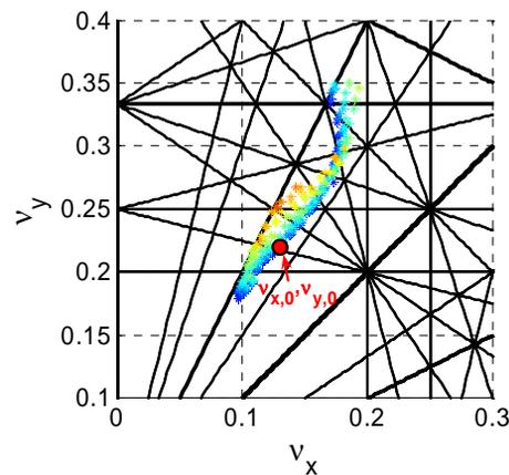
Figure 7: Measured  $(x_\beta, \Delta p/p)$  tune map, new optics, IDs open.
