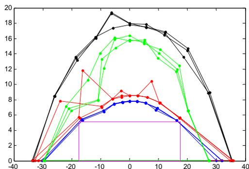
Fig. 4: Dynamic aperture for a single ID (Table 2). Black – bare lattice, green – DW, red – SCU, blue – MGU. Three random seeds are plotted for each ID.
