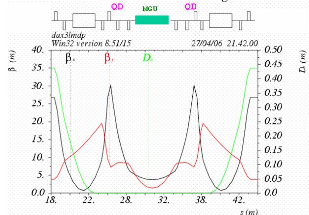
Fig. 1: One period of the NSLS-II lattice with a 3m MGU (green bar) shown, together with the quadruplets.
