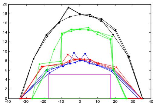
Fig. 5: Dynamic aperture for the set of 15 SCUs, 15 MGUs and 5 DW (Table 2)
