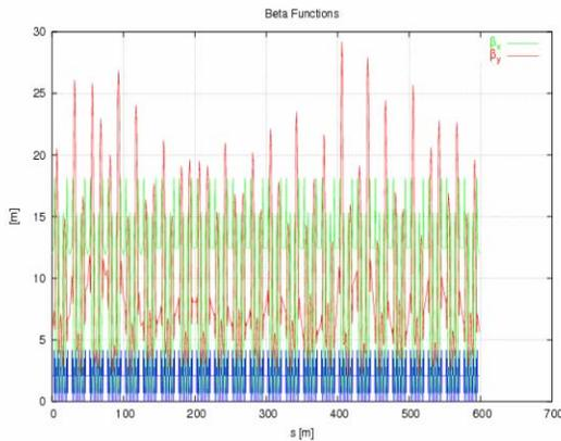
Fig. 2: Eighteen IDs with random field strength are included into the lattice
