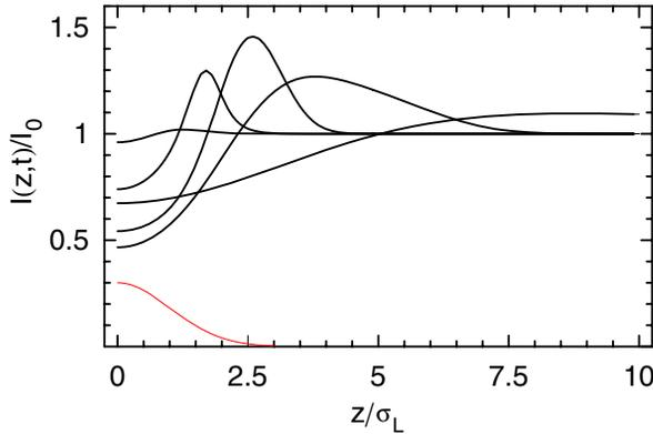
Figure 1: Density distributions at times  $ct\alpha/\sigma_L = 0.05, 0.2, 0.5, 1, 3$  (broader distributions correspond to later times) for  $A_0 = 6$ . The red curve shows the laser profile. The plot shows only positive values of  $z$ —the curves are symmetric about the value  $z = 0$ .
