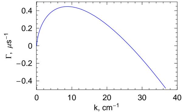
Figure 2: The growth rate of the CSR instability versus the wave number  $k$  for the ALS ring with  $\alpha = 2.7 \times 10^{-3}$ ,  $\sigma_\delta = 10^{-3}$ , and the average single bunch current of  $15 \text{ mA}$ .
