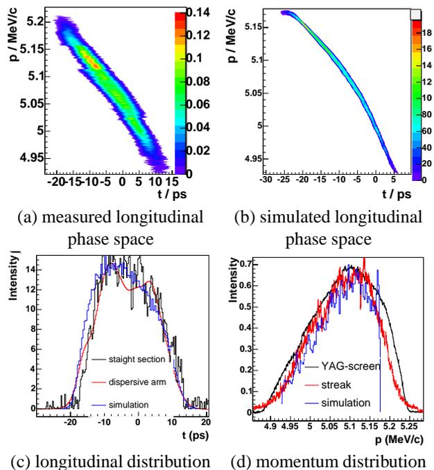
Figure 7: Measured (a) and simulated (b) longitudinal phase space and their projections: longitudinal (c) and momentum (d) distribution for 1.1 nC bunch charge, phase with maximum energy gain  $+10^\circ$  and a longitudinal laser distribution with about 20 ps FWHM pulse length. In (c) and (d) the black curves are direct measurements, the red ones are the projections of the measured longitudinal phase space and the blue ones are ASTRA simulations.
