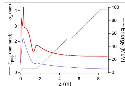
Figure 1: Transverse normalized emittance, radial spot dimension and energy along the photoinjector beamline for the medium bunch regime.
