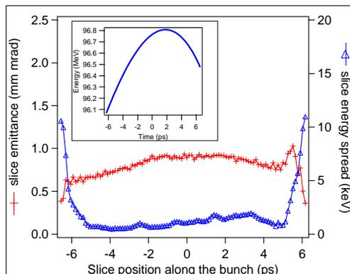
Figure 2: Slice emittance and slice energy spread at the injector exit for the medium bunch case. Inside plot: Longitudinal phase space including longitudinal wakefields. Bunch head is on the left.
