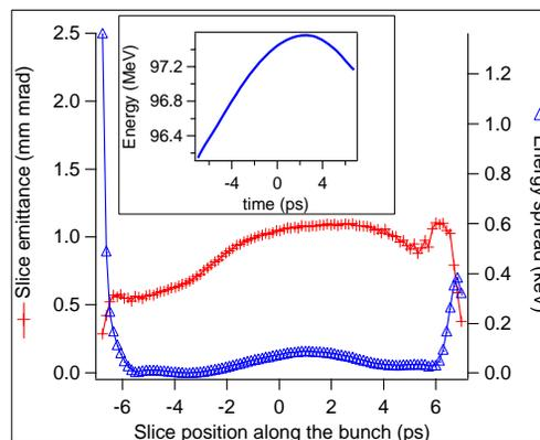
Figure 3: Slice emittance and slice energy spread at the injector exit for the long bunch case.
