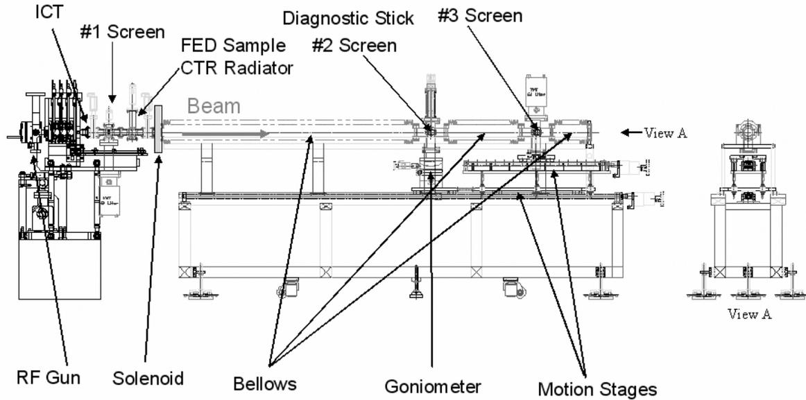
Figure 1: Schematic diagram of experimental setup of the gun test stand (GTS) for photo-injector developments of the PAL-XFEL.
