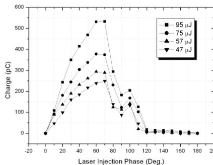
Figure 5: Laser injection phase vs photo electron charge depending on the laser beam energy.
