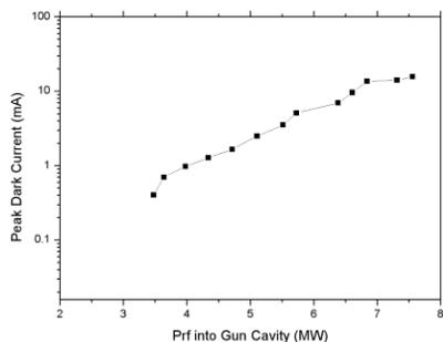
Figure 4: RF power into the gun cavity vs peak dark current.
