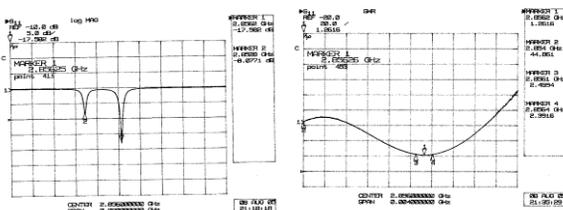
Figure 2: Cavity parameters using HP 3510C Network Analyzer. S11 parameter (left), standing wave ratio (SWR) representation of the cavity (right).
