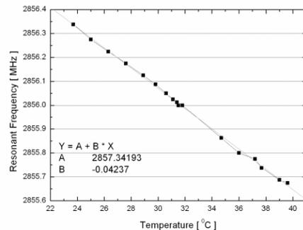
Figure 3: Measured temperature coefficient of the cavity. The temperature coefficient is measured as - 42.37 kHz / °C.
