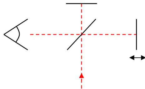
Figure 2: Principle of a Michelson Interferometer. A pulse enters, is split by the beam splitter, travels the different lengths to the mirrors and is recombined again at the beam splitter, and finally viewed with the detector.
