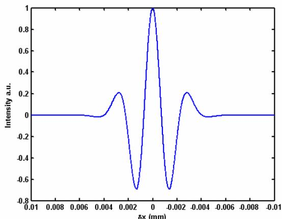
Figure 5: Autocorrelation of the radiation from a Gaussian electron beam.
