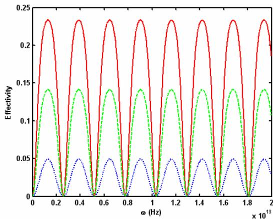
Figure 3: Beam splitter effectiveness for a 254  $\mu\text{m}$  Hostaphan foil. The solid red line is for transversely polarized radiation, the dotted blue for longitudinally polarized and the dashed green is an average.
