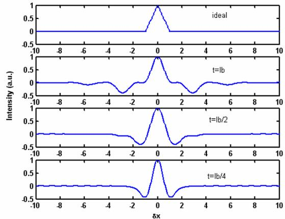
Figure 4: Expected signals if a square pulse of width  $lb$  FWHM goes through a Michelson interferometer with a beam splitter that is, from above: ideal, a foil with thickness  $t=lb$ ,  $t=lb/2$ ,  $t=lb/4$ .  $\delta x$  is in units of  $lb$ .
