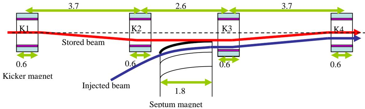
Figure 1: Schematic layout of the TPS injection system, in units of m.
