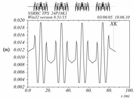
Figure 7: Horizontal required aperture acceptance of the TPS storage ring of  $\pm 4\%$  momentum deviation, lattice 24P18K1.
