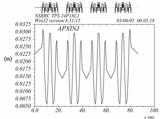
Figure 2: The aperture acceptance required at injection in the horizontal plane of TPS storage ring.
