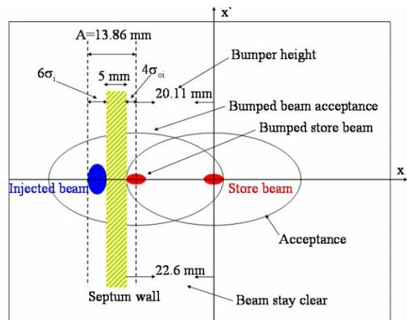
Figure 3: Horizontal phase space at the injection point.
