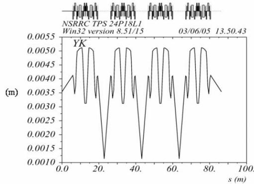
Figure 6: Vertical required aperture acceptance of the TPS storage ring of  $\pm 4\%$  momentum deviation, lattice 24P18L1.
