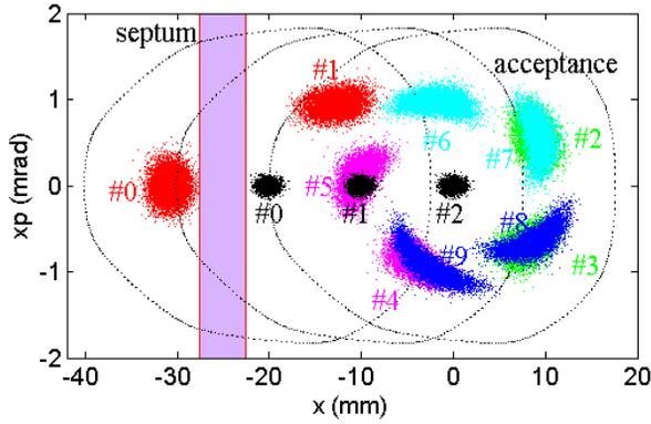
Figure 4: Horizontal phase space tracking of injected beam for the first few turns.
