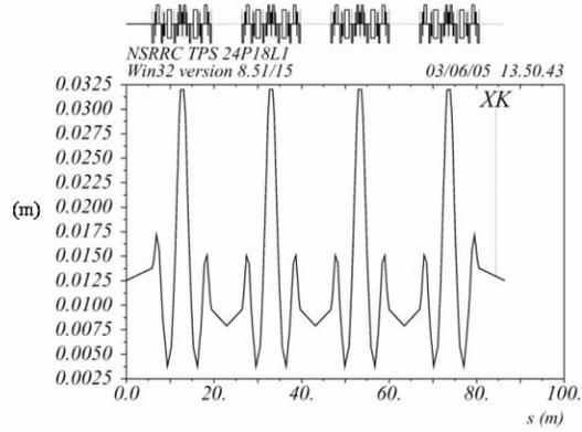
Figure 5: Horizontal required aperture acceptance of the TPS storage ring of  $\pm 4\%$  momentum deviation, lattice 24P18L1.
