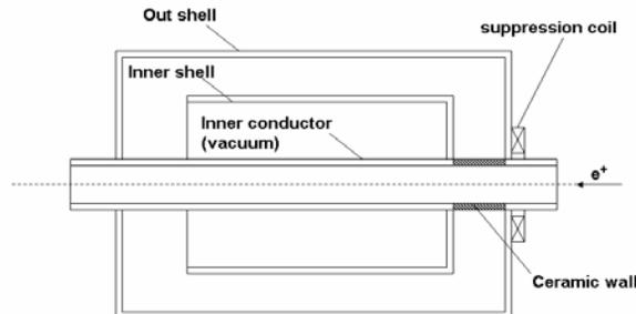
Figure 1: Schematic of the fundamental cavity.
