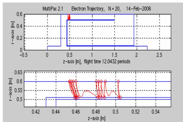
Figure 4: Simulation result with MULTIPAC. The top plot shows the location of a possible multipacting spot. The bottom trace is an expanded view of the spot area.
