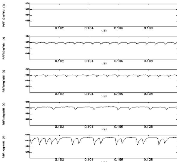
Figure 3: Expanded views of the scope traces. The falling edges are gap voltage drops at the start of a multipacting cycle and the trailing edges are at the recovery of gap voltage after a cycle.
