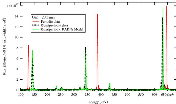
Figure 7: Flux calculated from measured and calculated magnetic fields for the FOM undulator at 23.5 mm gap.
