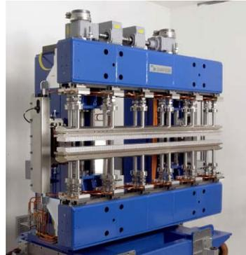
Figure 1: The SLS undulator without vacuum chamber.
