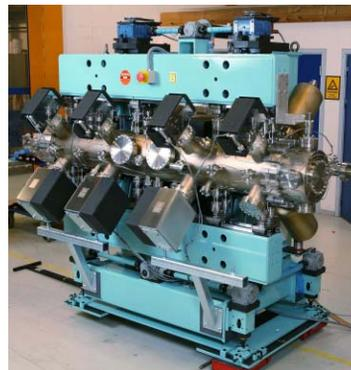
Figure 2: The SOLEIL undulator with vacuum chamber.
