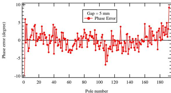
Figure 4: Phase angle error at 5 mm gap for the SLS undulator.
