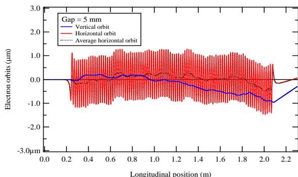
Figure 3: The horizontal and vertical electron trajectory as calculated at 5 mm for the SLS undulator.
