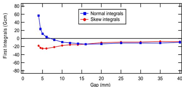
Figure 5: Measured gap dependence of the normal and skew first integrals for the SLS undulator.
