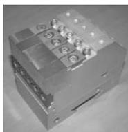
Figure 4: Five magnets module prototype for the further 52 mm period APPLE-II type undulator.
