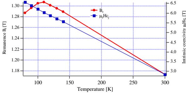
Figure 2: Measured intrinsic coercivity and remanence for NdFeB material versus temperature.
