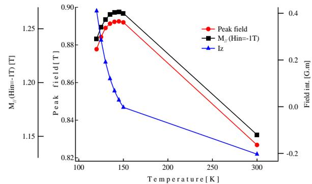
Figure 5: U18 peak field and on-axis vertical field integral versus temperature (blue) for a gap of 6 mm.
