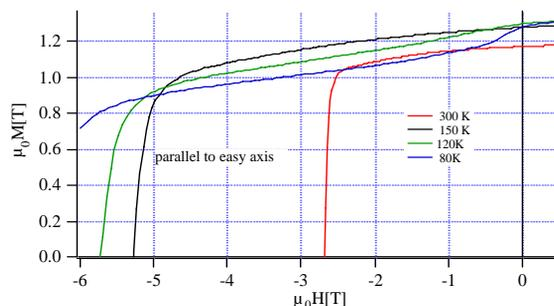
Figure 1: Recoil curves for NdFeB material at different temperatures.
