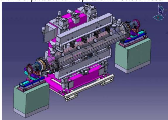
Figure 7: Schematic view of the measuring bench with its vacuum chamber.
