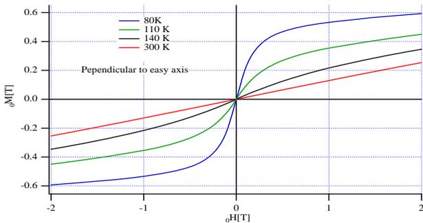
Figure 3: Measured magnetization perpendicular to the easy axis for different temperatures.
