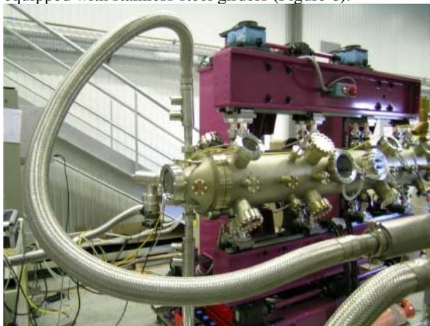
Figure 6: ESRF in-vacuum structure under cryogenic tests.
