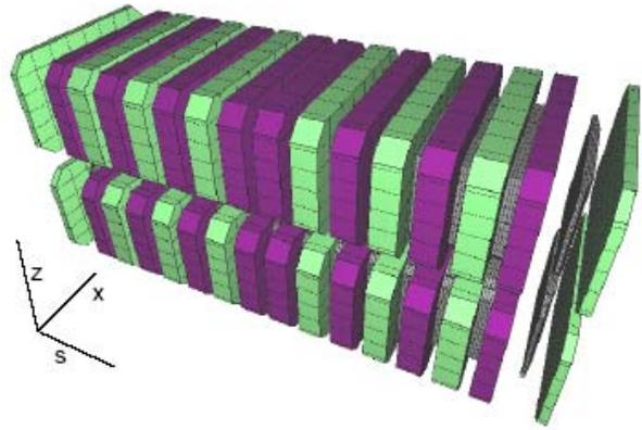
Figure 4: Hybrid undulator with end field termination adopted at the ESRF modelled in RADIA.
