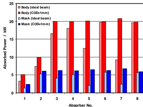
Figure 6: Power load on the body and mask part of the regular absorbers.
