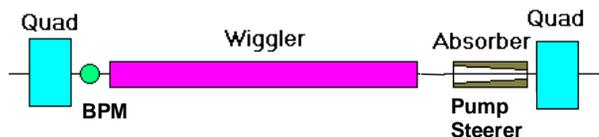
Figure 1: Layout of a regular cell in the damping section.
