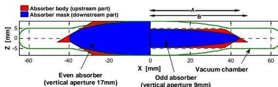
Figure 5: General layout of the absorber cross sections for the 2 types of odd and even regular absorbers. The wiggler vacuum chamber cross section is shown for comparison.
