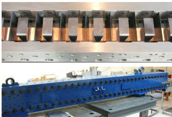
Figure 2: Pre-assembled wiggler half before insertion of magnets (top) and completed 4m long prototype (bottom).
