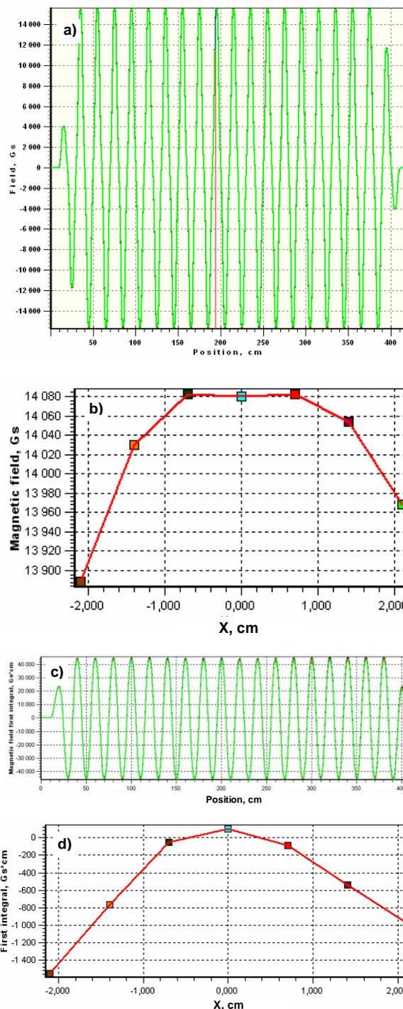
Figure 3: First Hall probe results of the long prototype: a) longitudinal field dependence, b) transverse field profile, c) 1st field integral, and d) its transverse distribution at the end of the structure (without finger correctors).
