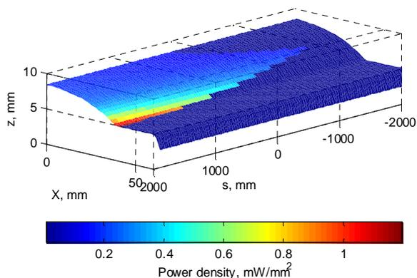
Figure 4: Power density distribution across the wiggler chamber (one quarter is shown).
