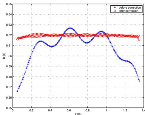
Figure 5: Maximum/minimum field values of the SCU model (III) with correction coils before and after correction with individual correction currents per period. The undulator model parameters are:  $n = 100$ ,  $g = 8$  mm,  $\lambda_u = 14$  mm and  $J_U = 900$  A/mm<sup>2</sup>.
