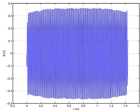
Figure 2: Magnetic field of the SCU14 installed at ANKA. The measurement was performed with a Hall-probe in a liquid helium bath [5]. The undulator parameters are:  $n = 100$ ,  $g = 8$  mm,  $\lambda_u = 14$ mm and  $J_U = 500$  A/mm<sup>2</sup>.
