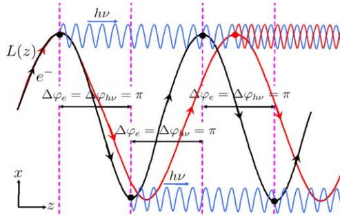
Figure 1: The variation of the period length or the amplitude of the magnetic field causes a slip between the electron phase and photon phase. In the worst case this leads to destructive interference.
