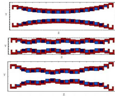
Figure 3: Schematic and strongly exaggerated drawing of the systematic mechanical distortions added to the Radia [10] model of a superconductive undulator: (I) bending (top), (II) periodical distortion (center) and (III) combination of both (bottom) [5].
