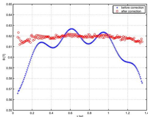
Figure 6: Maximum/minimum field values of the SCU model (III) with correction coils powered with four fixed currents before and after correction. The undulator model parameters are:  $n = 100$ ,  $g = 8$  mm,  $\lambda_u = 14$  mm and  $J_U = 900$  A/mm<sup>2</sup>.
