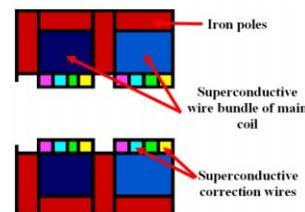
Figure 4: Wire allocation to the four correction coils in one period: Correction coil one (purple) with the current density  $J_{c,1}$ , correction coil two (turquoise) with the current density  $J_{c,2}$ , correction coil three (green) with the current density  $J_{c,3}$  and correction coil four (yellow) with the current density  $J_{c,4}$ .
