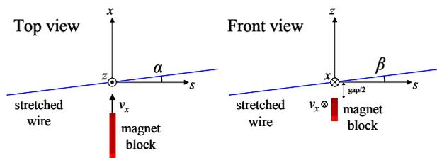
Figure 3: Misalignment angles of the stretched wire relative to the direction of displacement of the magnet block.
