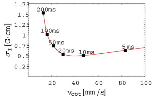
Figure 2: Dependence of the *rms* error in the determination of the field integrals ( $\sigma_I$ ) to the optimum velocity ( $v_x$ ) for different values of the integration window ( $\tau$ ), corresponding to a fixed stretched wire with  $N = 10$ .
