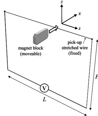
Figure 1: Sketch of a fixed stretched wire system.
