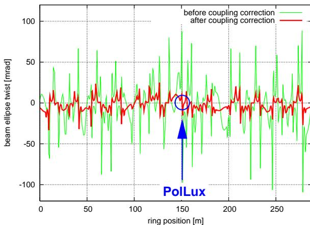
Figure 3: Twist of the electron beam ellipse as a function of the longitudinal SLS storage ring position for a  $-300 \mu\text{rad}$  steering for the PoILux beamline before (green line) and after (red line) betatron coupling correction. The twist has been determined from the calculation of generalized sigma matrices [5] within the computer code TRACY [6]. The arrow denotes the location of the 4-bump for the PoILux beamline.
