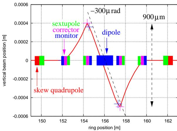
Figure 2: Layout of the vertical asymmetrical “polarization” bump consisting of four successive dipole correctors (magenta bars) for the dipole (thick blue bar) beamline PoILux. Dedicated skew quadrupoles (red bars) are foreseen to locally compensate for the betatron coupling induced by the sextupoles (green bars) within the bump.
