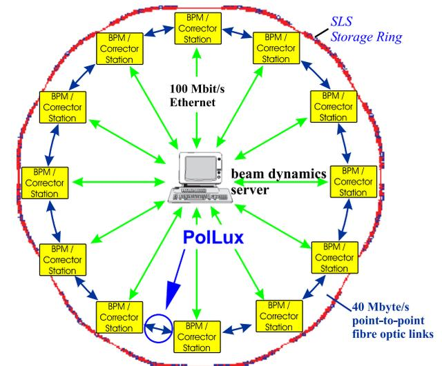
Figure 4: The global fast orbit feedback (FOFB) is integrated in 12 beam position monitor (BPM)/corrector sectors (stations) [2]. The start of the execution of the feed forward (FF) table, which will be implemented as part of the FOFB system has to be synchronized between two FOFB processor boards since the boundary of two sectors is just across the PoILux bending magnet (blue circle).
