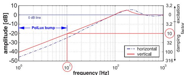
Figure 6: FOFB closed loop transfer function in the horizontal (blue dashed line) and vertical (red line) plane at the SLS [7]. It should be feasible to achieve polarization switching rates of up to  $\approx 10$  Hz for mostly sinusoidal waveforms with flat tops of variable length at  $\pm 300 \mu\text{rad}$ .
