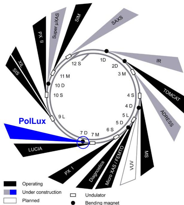
Figure 1: Schematic layout of the Swiss Light Source (SLS). The new microspectroscopy beamline PolLux (blue fan) is located in the arc of sector 7 employing the light emitted by a central  $14^\circ$  bending magnet (blue circle).
