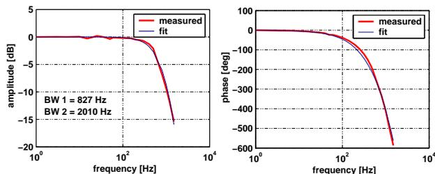
Figure 5: Vertical open loop transfer functions of the global fast orbit feedback (FOFB). The model of the fit consists of a series of a first (bandwidth (BW) 1) and fifth order (BW 2) low pass filters and a time delay [8].
