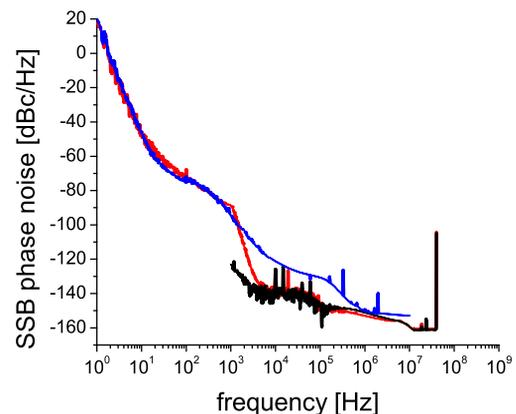
Figure 3: Spectral density of single-sideband phase noise for the free-running EDFL (black), the RF reference oscillator used to lock the EDFL (blue), and the EDFL locked to the reference (red).
