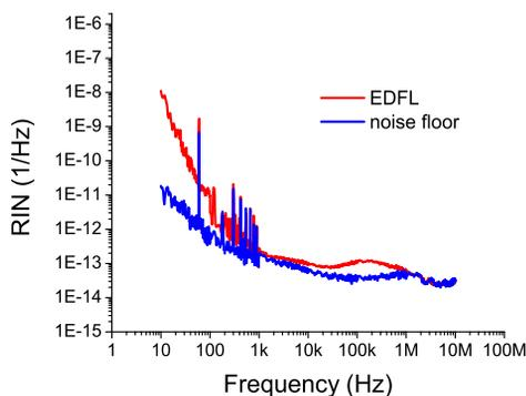
Figure 4: Relative intensity noise (RIN) of the EDFL, along with the measurement noise floor.
