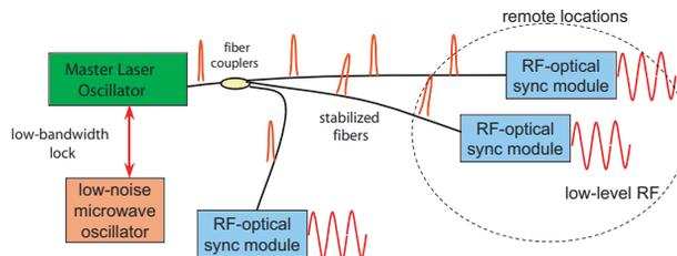
Figure 1: Schematic of the optical timing synchronization system.
