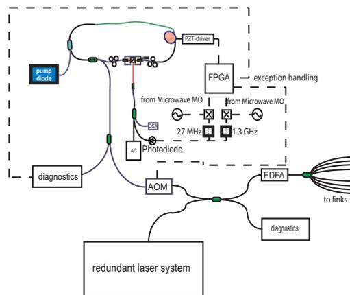
Figure 7: Schematic of the LMO System for the FEL facility FLASH at DESY
