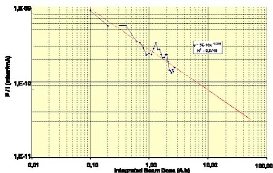
Fig.5: Average pressure of Cell C07 normalised to current vs integrated beam dose.
