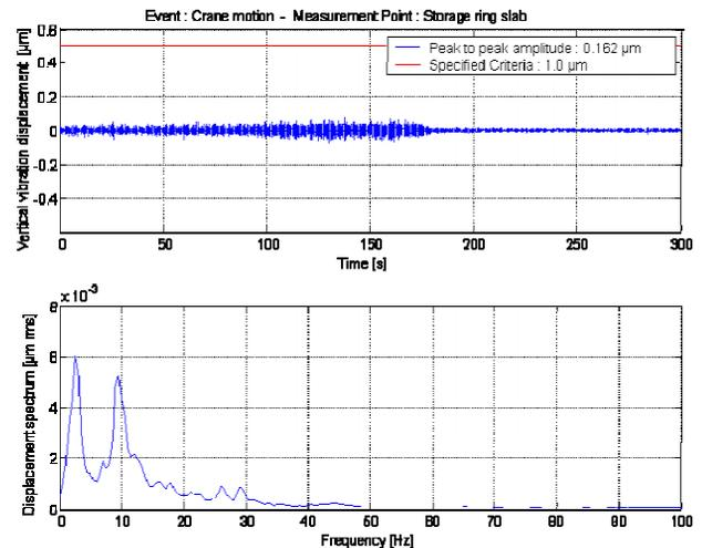
Fig.1: Vibrations induced on the SR slab during crane motion.
