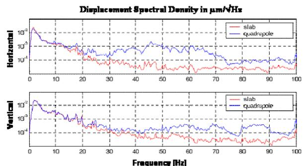
Fig.2: Displacement spectral density recorded on a SR quadrupole magnet after final installation in the tunnel.
