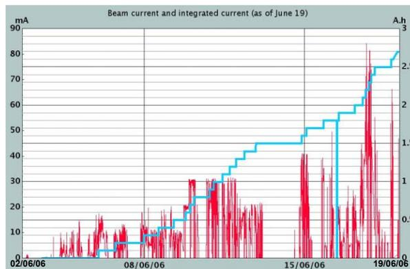
Fig.4: Beam current (red) and evolution of the integrated current (blue) during the 3 week run.
