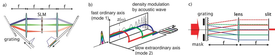
Figure 3: Scheme of different techniques for longitudinal pulse shaping of laser pulses: a) dispersion free pulse-shaper using a spatial light modulator, b) acousto-optic programmable dispersive filter and c) direct space-to-time pulse-shaper.
