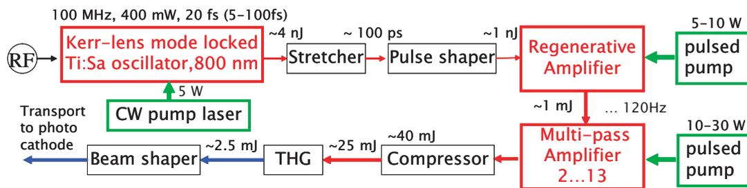
Figure 1: Typical layout of photocathode laser system for Cu-cathodes.
