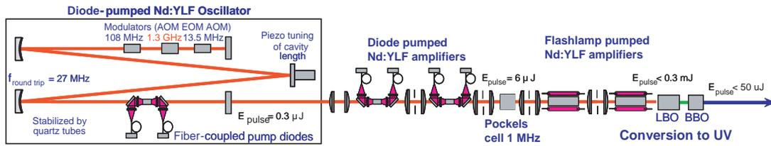
Figure 2: Photocathode laser system of FLASH.
