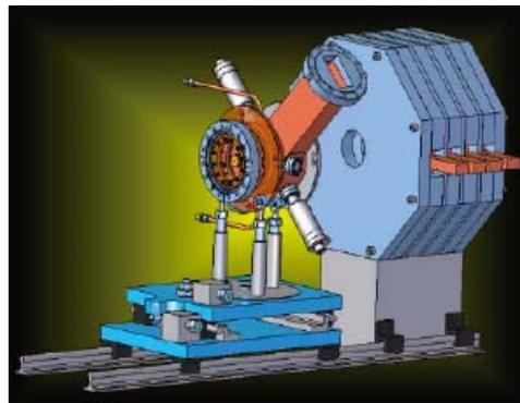
Figure 4: 1.6 cells S-band gun cavity of the BNL/SLAC/UCLA design with solenoid.
