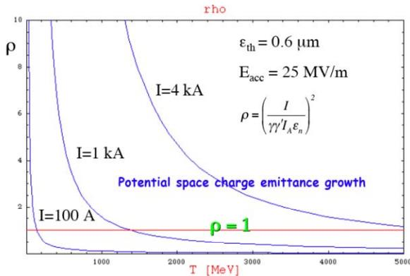
Figure 2: Laminarity parameter  $\rho$  versus beam energy  $T$  for different beam currents. Notice for example that a 1 kA beam is space charge dominated up to 1 GeV.
