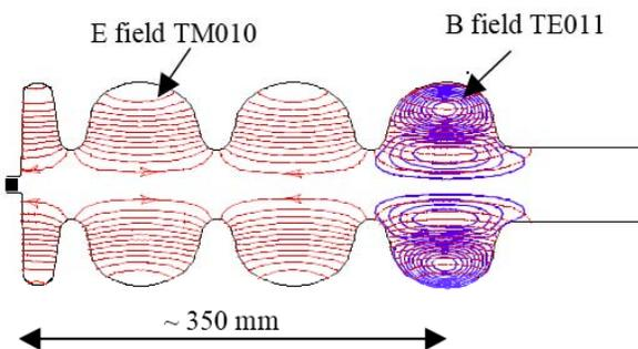
Figure 7: Electric field of the accelerating TM010 mode (red lines) and magnetic flux of the solenoidal TE011 mode in 3.5-cell L-band superconducting FZR cavity.
