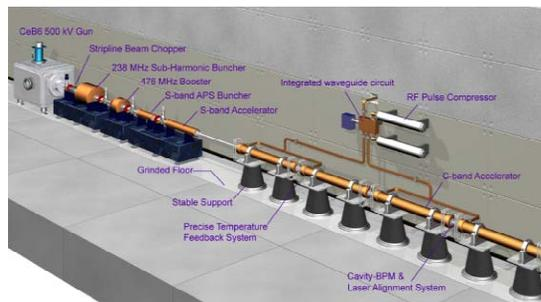
Figure 6: Layout of the SCSS thermionic injector.
