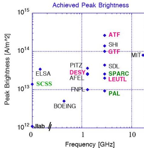
Figure 3: Achieved peak brightness versus gun frequency. Red labels: results achieved with  $\rho < 1$ , black labels: measurements performed at low energy  $\rho > 1$ , green labels: preliminary results of new facilities. DC guns are indicated as 0 frequency.
