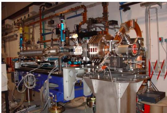
Figure 5: 1.6 cells S-band gun cavity with solenoid and movable emittance meter installed in the SPARC hall.
