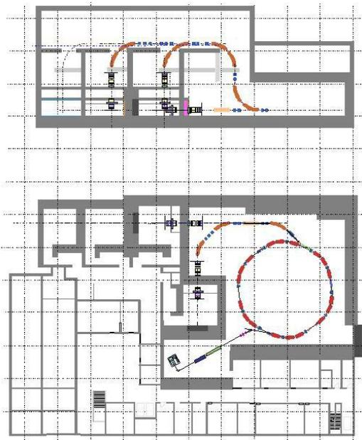
Figure 5: Layout of new carbon-therapy facility at Gunma University.
