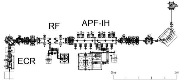
Figure 3: A test bench for the compact injector system.
