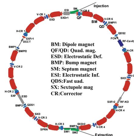
Figure 4: Layout of synchrotron.
