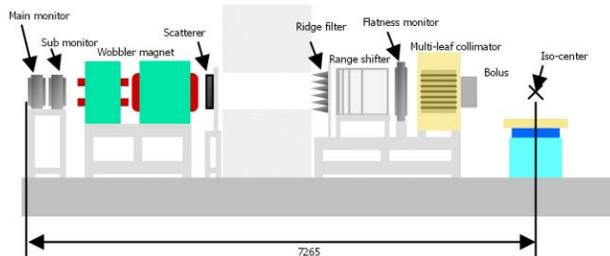
Figure 1: Layout of the beam delivery system.
