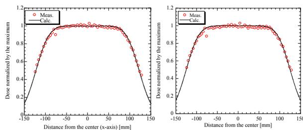
Figure 2: Lateral dose distribution by spiral wobbler (left) and raster scanning (right) after 1 min irradiation. Circles are measured dose distribution and solid line designed one.
