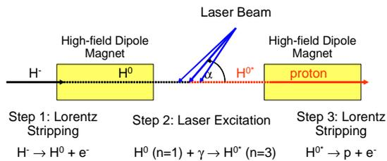
Figure 1 General scheme of frequency sweep stripping.
