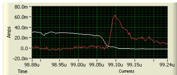
Figure 4 Ion beam current (white line) and the signal from photodiode (red line). One can see the dip in the beam current 200 ns from the end of the pulse.
