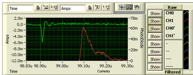
Figure 5 Proton beam signal (green line), shifted forward 200 ns relative to the photodiode signal (red line).
