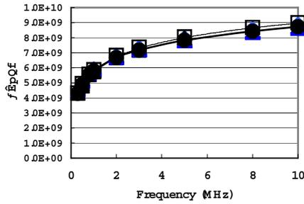
Figure 2:  $\bar{\mu} Qf$  mean values of cores in each group with three cores.
