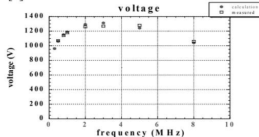
Figure 5: Obtained acceleration voltages ( $\square$ ) with input-power of 2 kW. The calculated values ( $\bullet$ ) are shown also.
