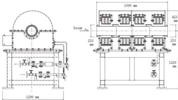
Figure 3: Left figure is cavity view from upstream, and the right figure is the cross-section of the cavity.
