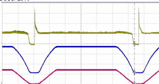
Figure 8: DCCT signal divided with acceleration frequency (upper), level signal of acceleration frequency (lower), and current pattern of dipole magnets. Horizontal scale is 0.5sec/div.
