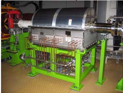
Figure 6: Acceleration cavity installed in the HIMAC synchrotron.
