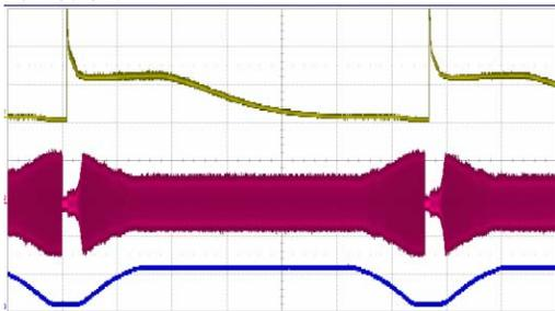
Figure 7: DCCT signal divided with acceleration frequency (upper), gap rf signal (middle), and level signal of acceleration frequency (lower). Horizontal scale is 0.5sec/div.
