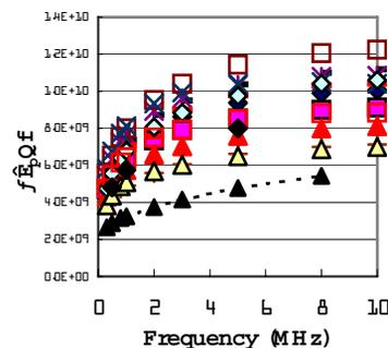
Figure 1:  $\bar{\mu}Qf$  values of twelve cores in the required frequency range. The symbol of  $\blacktriangle$  show the values of FINMET FT-3M.
