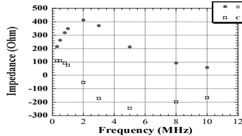
Figure 4: Cavity impedances of the quarter wave resonator as a function of the rf frequency. The real part ( $\bullet$ ) and the imaginary part ( $\square$ ) of the impedances are shown together.
