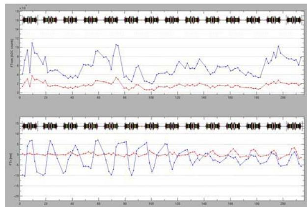
Figure 1: First turn without injection kickers. The horizontal axis is the  $s$  position of the BPM. Top: shows the sum signal, the variation in strength comes from cable attenuations. Bottom: first turn horizontal orbit.
