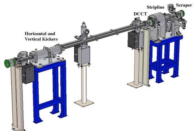
Figure 5: The diagnostic straight includes the kickers, DCCT, stripline and scraper.
