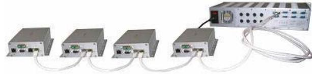
Figure 3: The BLM measurement system consists of an IOC and 14 counters each with 1 BLM.
