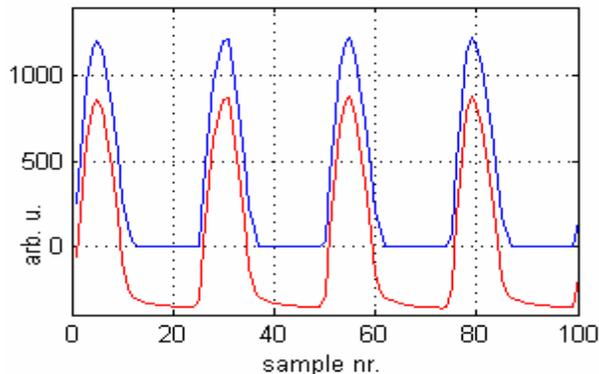
Figure 5: Blue curve: signal after baseline restoring, red curve: original PU signal.
