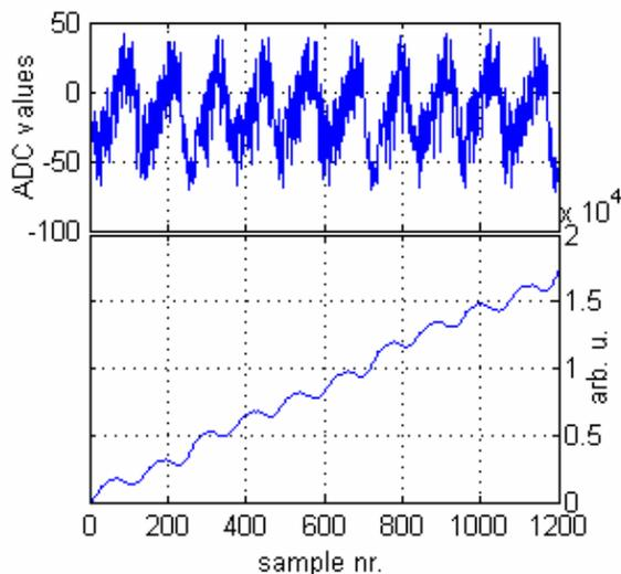
Figure 1: Top curve: original PU signal, bottom curve: accumulated and filtered PU signal.
