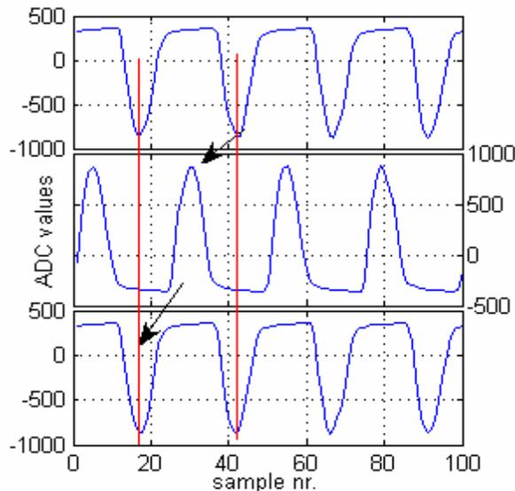
Figure 4 Top curve: inverted original signal, middle curve: original signal delayed by half an RF period, bottom curve: inverted original signal delayed by one RF period. The black arrows show the position of one particular bunch; the red lines mark the area of interest.
