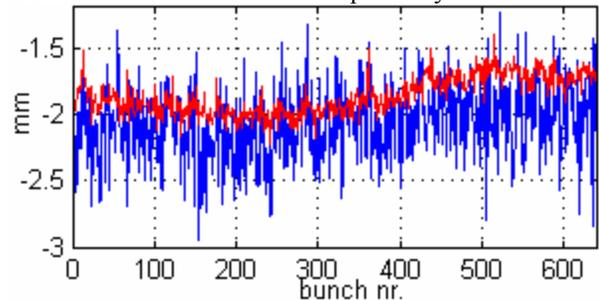
Figure 6: Calculated position over approx. 150 turns on harmonic 4, blue curve showing the results with linear BLR, the red curve showing results using the introduced BLR.
