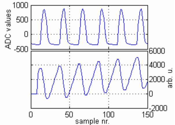
Figure 2: Top curve: original PU signal, bottom curve: accumulated and filtered PU signal
