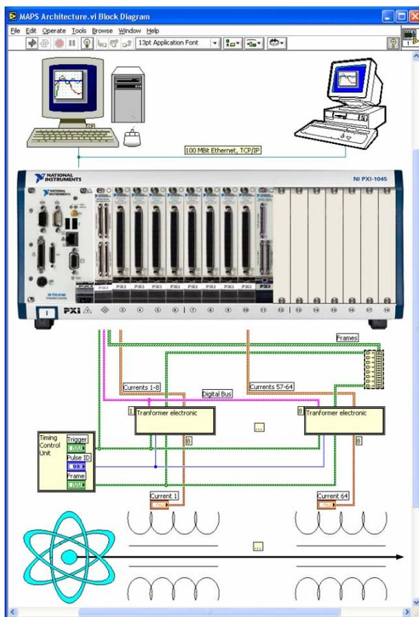
Fig. 3 Architecture of the upgraded system [4]
