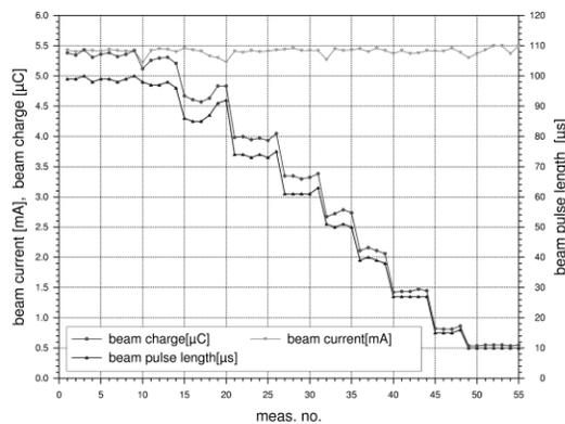
Fig. 2 Beam-pulse charge and length (see Fig.1)
