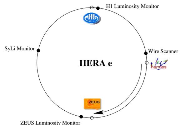
Figure 1: Location of profile monitors in the HERA electron ring together with the high energy physics experiments ZEUS, H1 and HERMES.
